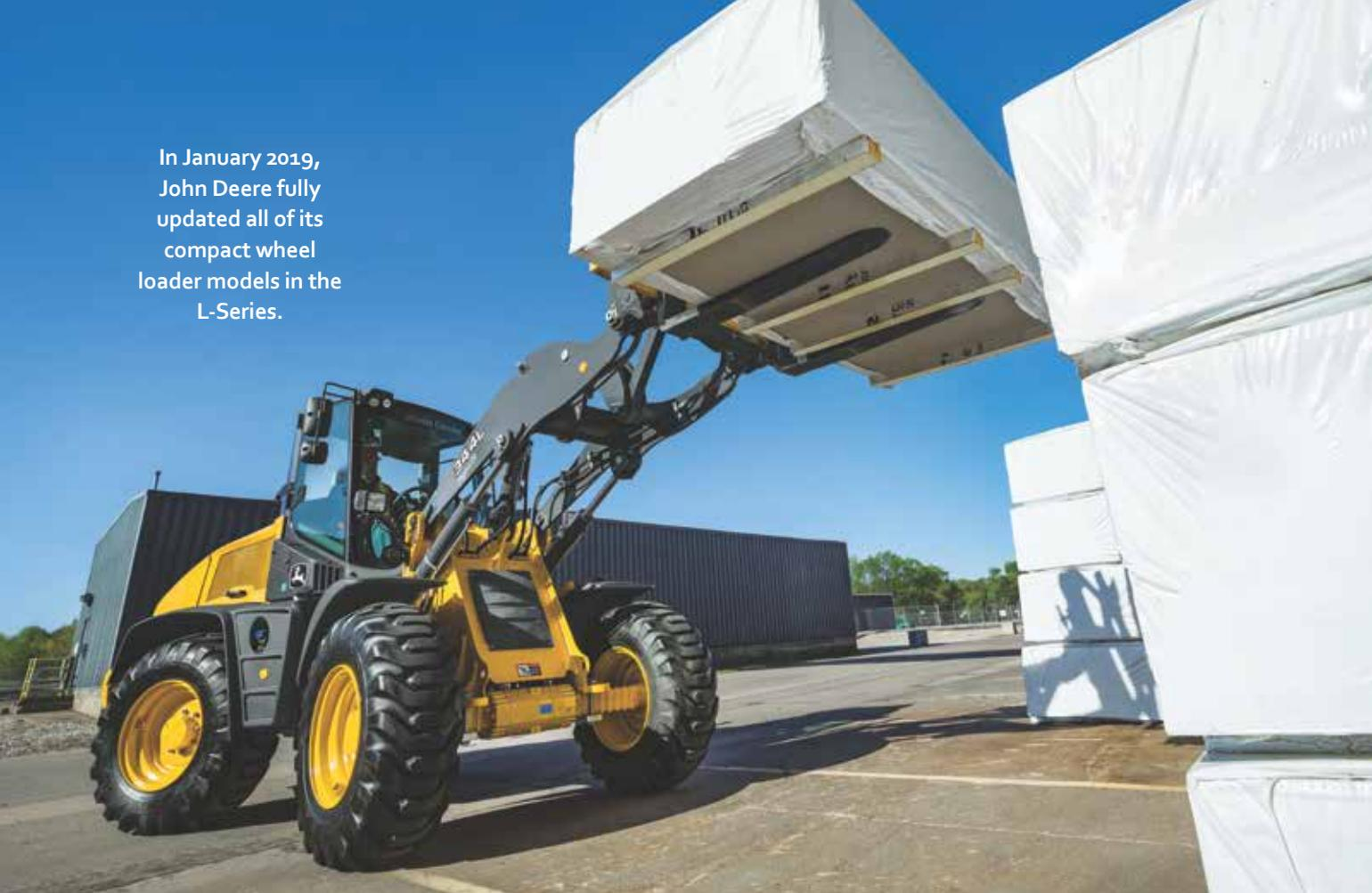
hydrostatic transmission with automatic shifting that has a top speed of approximately 23 to 25 mph [depending on the model].”
